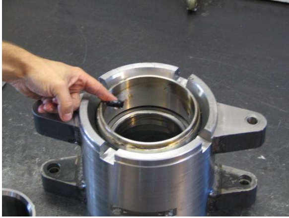
Flip the Chuck Housing over and apply grease to the inside surface of the Piston
