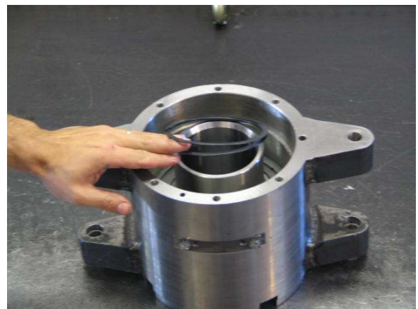
Flip the Chuck Housing over. Install the Retaining Ring (18100406)
