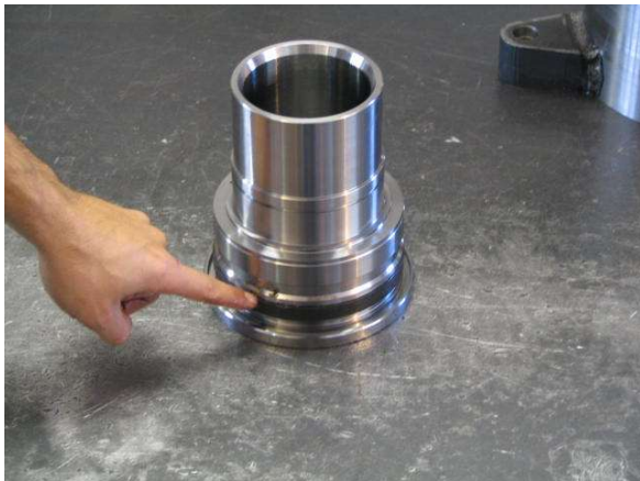
Apply grease to the outside surface of the Wear Ring.
