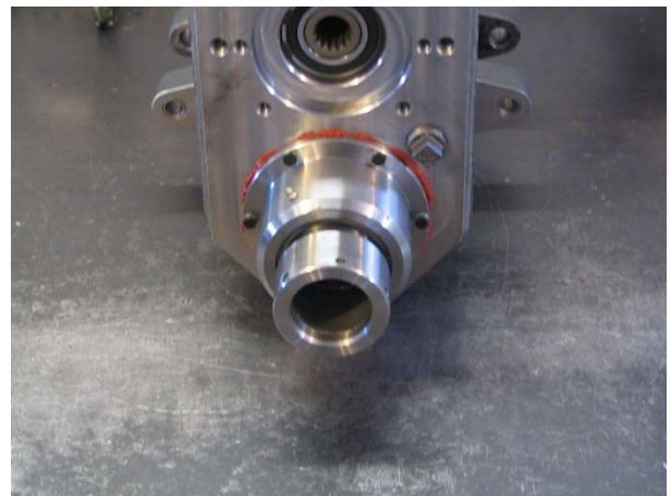
Apply an anti seize compound to the thread on the end of the Spindle, and screw on the Output Shaft Nut (18100513).
