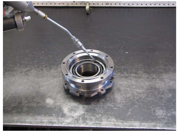
Apply grease the other side of the Ball Bearing
