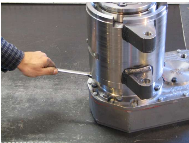
Insert the 8 bolts (3/8-24 x 1-1/2" HHCS) and Lock Washers to fasten the Chuck Housing to the Thrust Bearing Housing.
