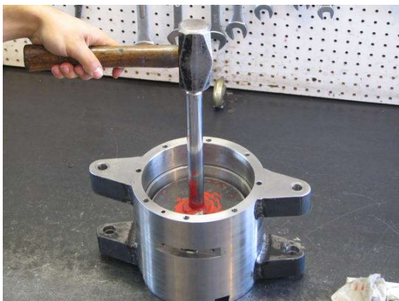
Hammer the Ball Bearing into place.
