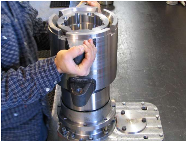
Install the Chuck Housing (18100343).
