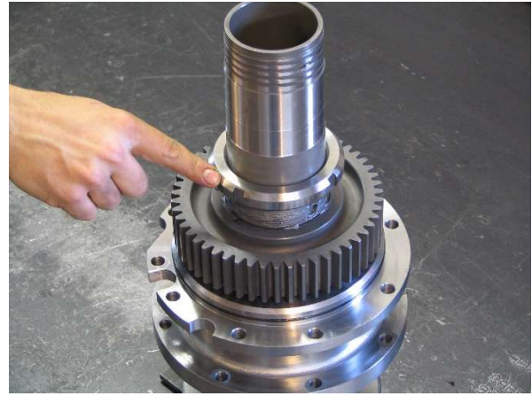
Install a Lock Nut (18100510) with the bevel facing up.
