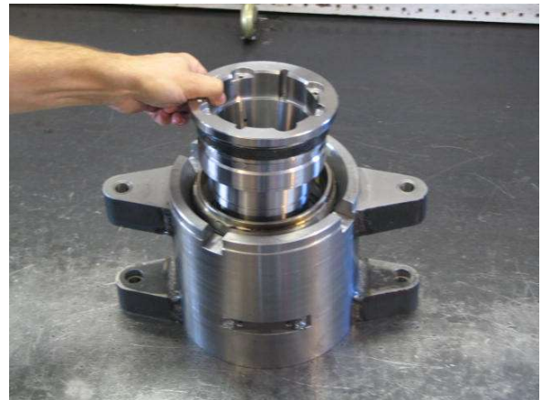
Flip the Chuck Bowl over and install it in Chuck Housing.
