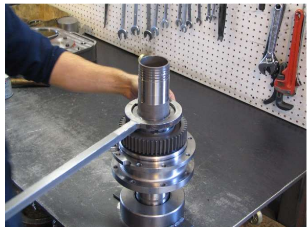
Tighten the Lock Nut.
