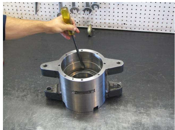
Ensure that the Retaining Ring is properly positioned in its groove in the Piston
