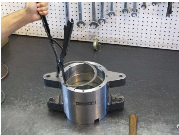
Use Retaining Ring Pliers to install
