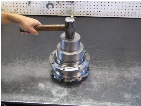
Hammer the Ball Bearing into place.
