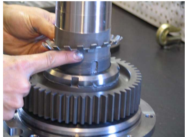
Install the Lock Washer (18100511) over top of the Nut. Ensure that the tab is lined up with the keyway in the Spindle.
