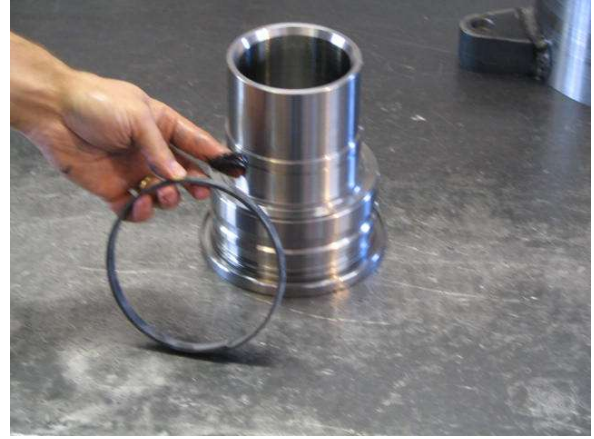
Install the Wear Ring (18100411) in its groove on the Chuck Bowl (18100419).
