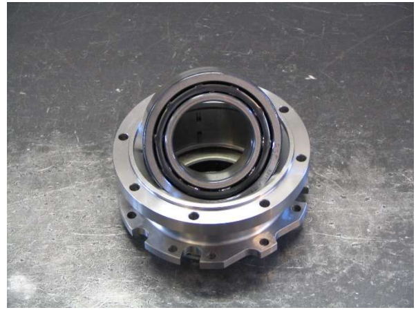
Flip the Ball Bearing over and install it in the Thrust Bearing Housing.
