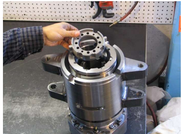
Use a Bushing to help properly align the Chuck Bowl and the Spindle, then position the Chuck Housing as shown.
