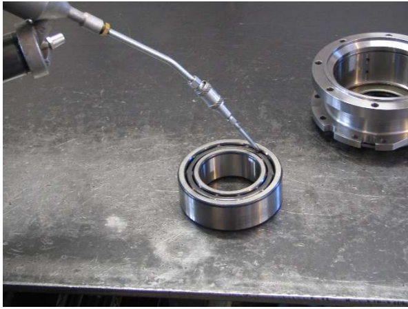
Apply grease to the Ball Bearing (18100410)
