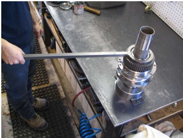
Tighten the Lock Nut. Spindle lock and lock nut wrench in grey cabinet. Bolt Spindle lock to table.
