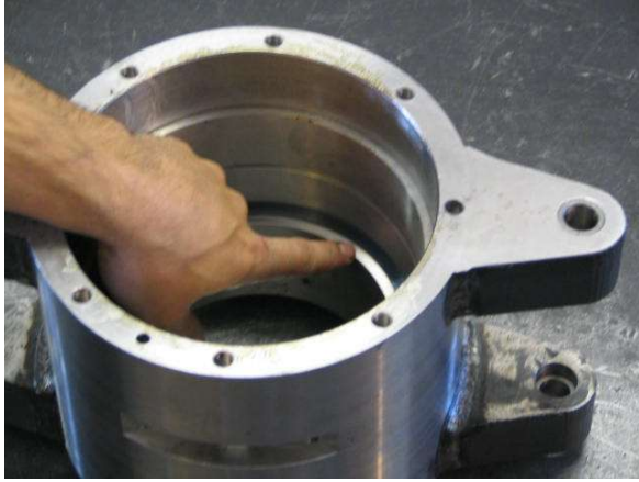
Ensure the Circlip is properly positioned at the bottom of the Piston.
