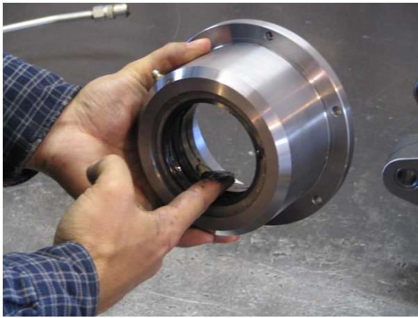
Apply grease on the Oil Seal and install over the Spindle. Fasten to the Drillhead Housing with the 6 Bolts (1/4" x 3/4" long) and the Lock Washers. Install 1" pipe plug.
