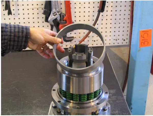
Install the Stop Tube (18100415).
