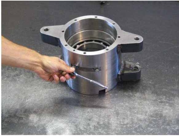
Install the 2 bolts (1/4" x 1/2" long) and the External Tooth Lockwashers.
