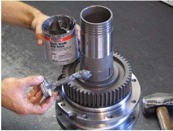
Apply an anti-seize compound to the thread on the Spindle
