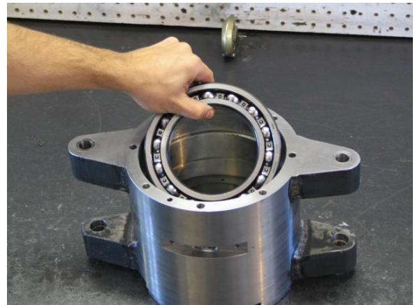
Flip the Ball Bearing over and install it in the Chuck Housing.
