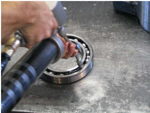
Apply a generous quantity of grease in the Ball Bearing (18100405)
