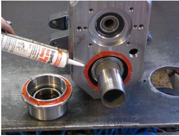
Apply silicone to the Drillhead Housing and the Upper Bearing and Seal Housing.
