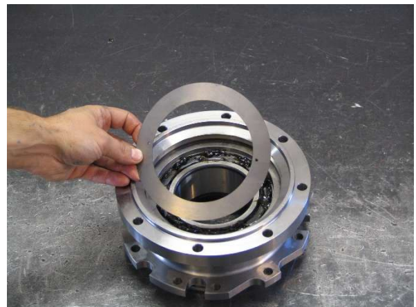
Install the Bearing Shield (18100409)
